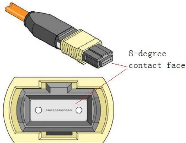
**Figure 6. Female MPO Connector with 8-degree End-face**
