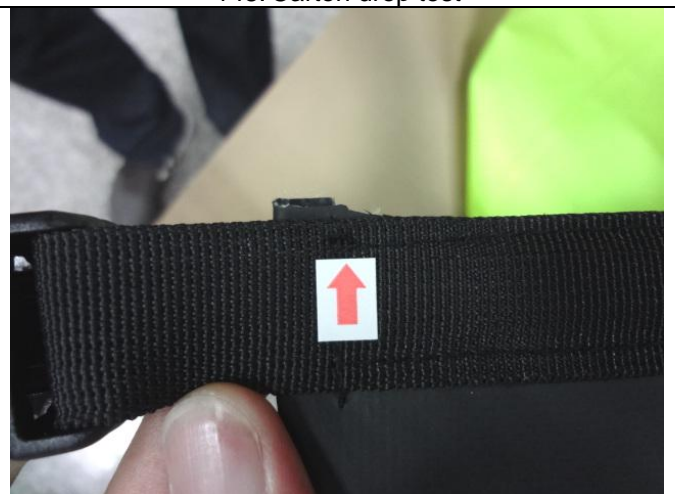
150. Defect: SE-2005-BLK -Poor cutting (minor)
