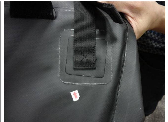
152. Defect: SE-2050-BLK- misaligned matched (major)
