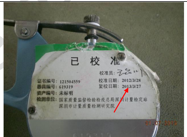
Expire date on thickness gauge
