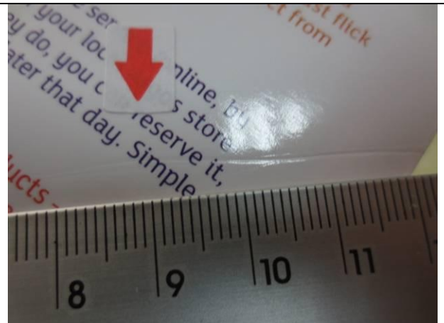
56. Minor defect: Obvious scratch mark on cardboard
