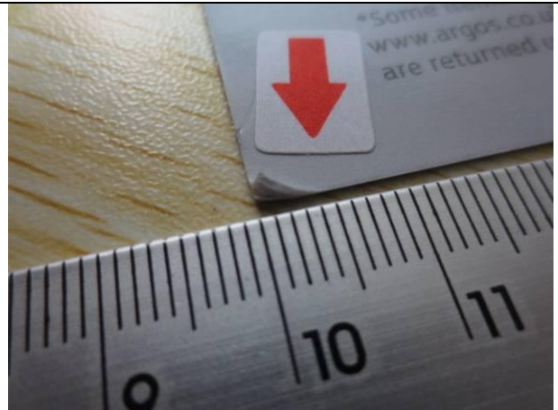
62. Minor defect: Frayed edge on cardboard
