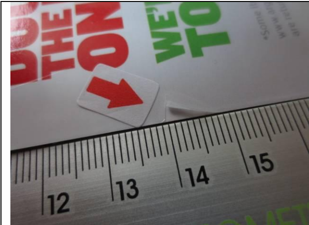
61. Minor defect: Frayed edge on cardboard
